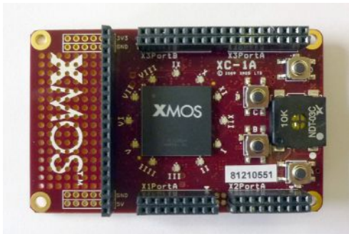
Figure 47: XMOS Development board XC-1A. Quad core processor 1,600 MIPS.
