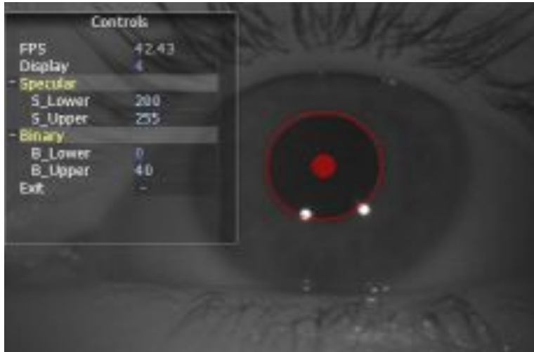
Figure 36: Pupil center detection in the capture routine. Still image of eye taken as screen capture of capture software.
